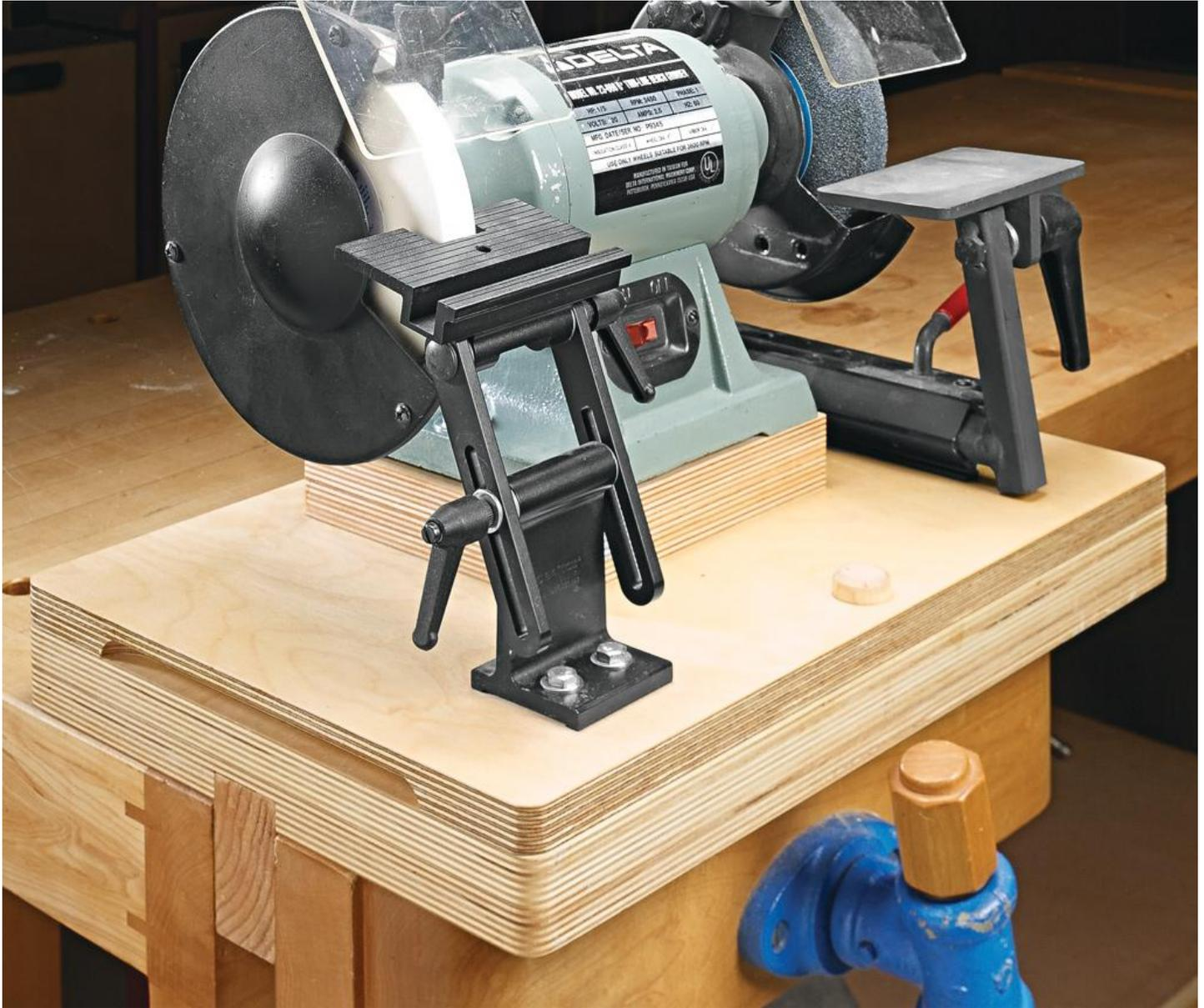
Workbench space is at a premium in my shop. To make the most of the space I do have, I wanted an easy way to use smaller bench-mounted tools (my grinder and machinist's vise) in the same location. What I came up with is this interchangeable work platform that clamps into the face vise on my bench.
