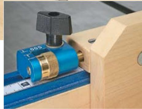
▲ **Box Joints.** You can easily turn the crosscut sled into a precise box joint jig with this commercial micro-adjuster.
