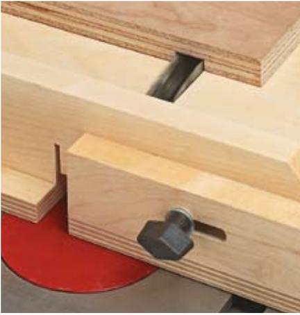
▲ **Zero-Clearance Base.** Whether you're making a simple crosscut or cutting dados, rabbets, or box joints, the adjustable base ensures less chipout.
