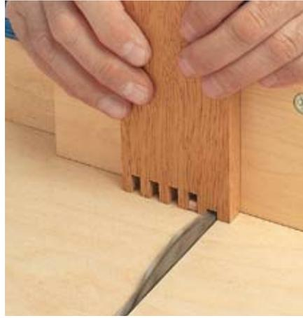
▲ **Add-On Accessories.** The versatile fence design allows you to easily add accessories like a featherboard, a stop block, or a box joint attachment.
