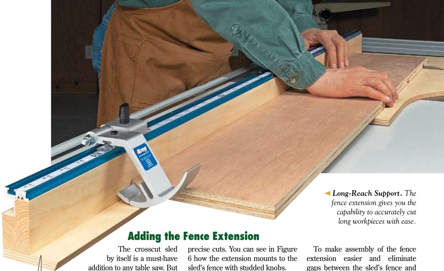
▶ **Long-Reach Support.** The fence extension gives you the capability to accurately cut long workpieces with ease.
