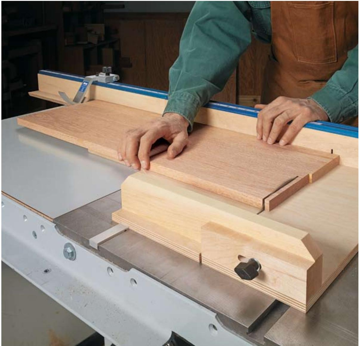
**W**hen crosscutting on the table saw, I like the fool-proof accuracy a sled provides. This solid but lightweight sled makes cutting long or wide workpieces easy.
