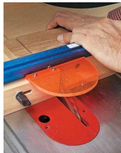
▲ **Blade Guard.** The guard helps keep your fingers away from the spinning blade as it exits the sled.
