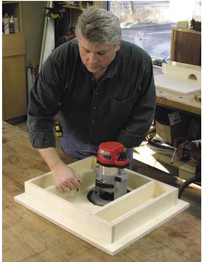
Allowing the proper clearance for your router is critical. You can see that I've removed the handles from the tool to allow as much space as possible. Mark out the space and then assemble the frame to fit.
