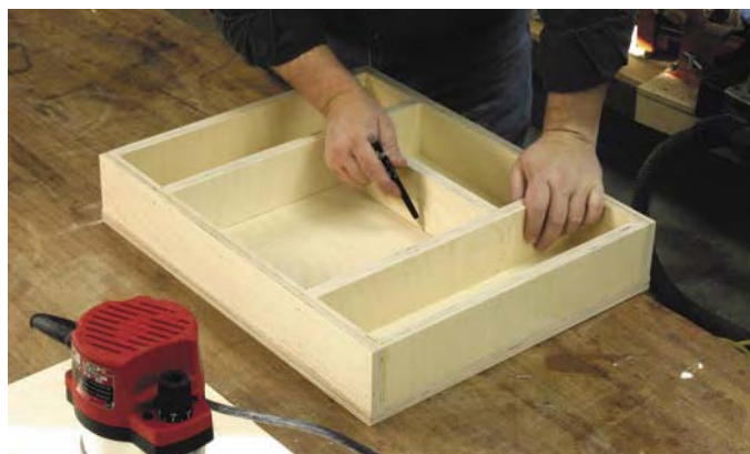
More marking: With the frame assembled and resting on the bottom piece, mark out the notch that will allow the router to extend through the top.
