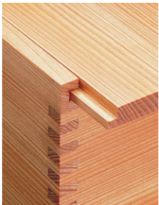
▲ The lid on this box slides into shallow grooves cut in the sides and back.
