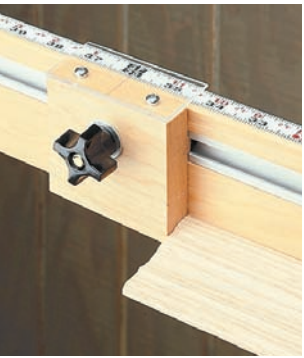
▲ To produce accurate results, this adjustable stop combines a sliding wood block with a plastic hairline indicator.
