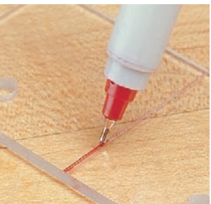
▲ To make the hairline stand out on the indicator, fill in the line with a permanent marker and then wipe off any excess.
