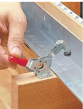
▲ Small toggle clamps make it easy to quickly adjust the position of the supports and fences.
