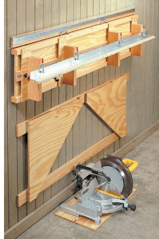
▲ After removing the miter saw, storing the station is just a matter of hanging it on a cleat and folding the supports for the station against the wall.
