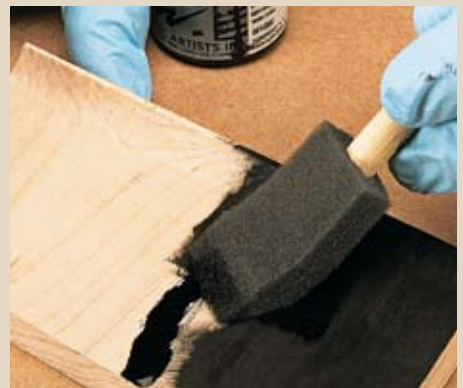
Then, with a disposable foam brush, you can spread the ink across the surface and work it into the grain as much as possible.
