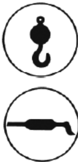
Hook up points for lifting unit and grease points
