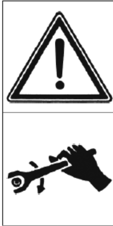
Always check bolts are well tightened
