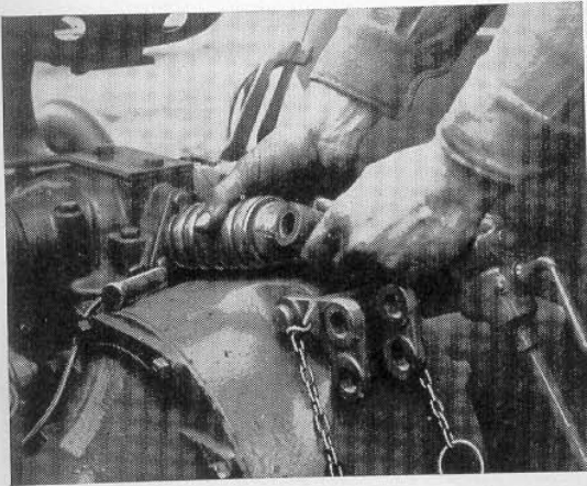
Fig. FO79—Adjust main control spring by rotating the threaded yoke as shown. Main control spring is listed as "lift draft control spring" in Ford parts catalog TIE 3731.
