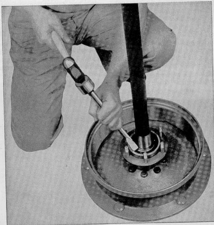
Fig. FO68—Removing the shrunk-on wheel axle shaft bearing retainer collar.
