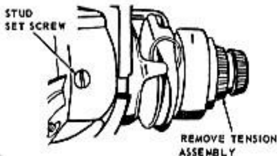
Fig. 30. Removal of Tension Assembly
