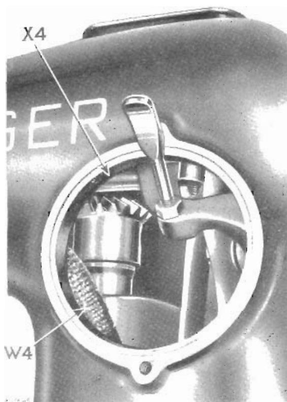
FIG. 11. STITCH INDICATOR PLATE REMOVED TO SHOW THE POSITION OF SINGERLIGHT LEADS IN THE ARM OF MACHINE 201 2
