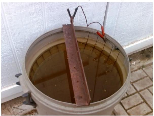
Some people have provided physical protection to prevent the sacrificial metal from touching parts. One of the best ideas I have seen was to cut a piece of 3/4" PVC pipe for each piece of rebar. Drill a series of large holes in the pipe about 1" apart and put the piece of rebar inside. The rebar can still "see" your parts through the holes, but the PVC helps keep them from actually touching.
