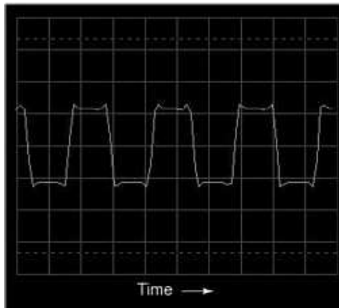
Figure 7.31: Oscilloscope time-domain display of a square wave
