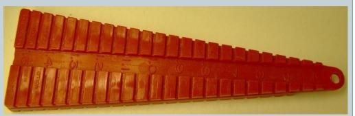
Hand-held resistor lead bending tool.
