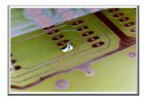
Figure 1.5: Good Solder Joint, [8]
