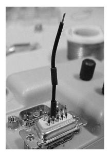
Figure 1.12: DB Connector with shrink wrap, [7]
