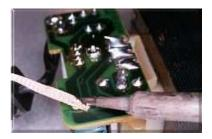
Figure 2.3: Desoldering with a Solder Wick, [8]
