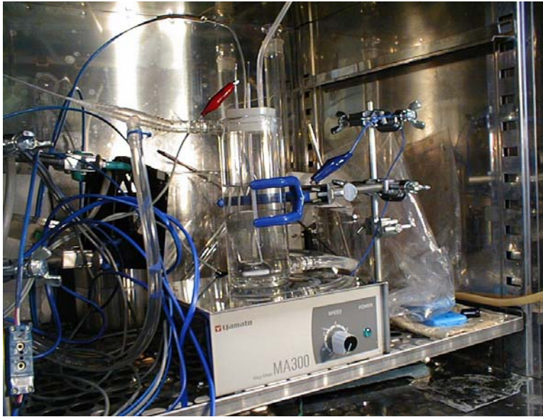
Figure 2.5. A glow discharge cell in climate-controlled cabinet in Mizuno's laboratory. Photo by J. Rothwell.
