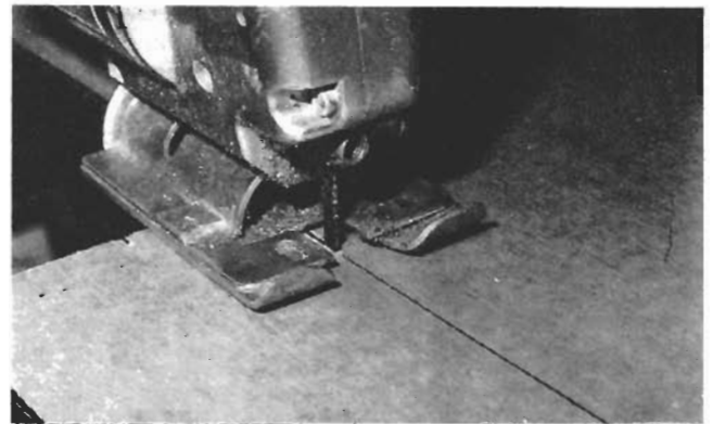
FIG. 4—THE BEST WAY to cut acrylic plastic is with an ordinary power saw, as shown here.
