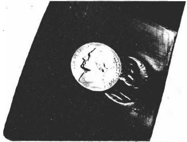
FIG. 7—IF YOU SOFTEN THE PLASTIC with solvent cement, you can emboss any designs you wish into the surface.
