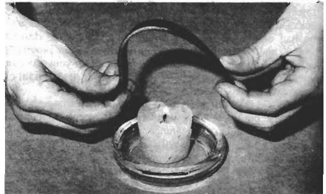
FIG. 3—ACRYLIC PLASTIC CAN BE EASILY BENT into any shape, if it's heated.
