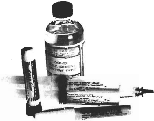
FIG. 2—ALL OF THESE GLUES will work with acrylic plastic, but the solvent cement is best for joining two pieces of plastic.
