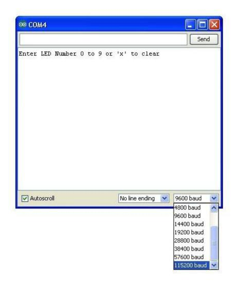
You should find that that everything still works. High speed communication not often necessary, so the baud rate of 9600 is often used, as many serial peripherals such as GPS modules will have this as a default baud rate, so it is something of a standard.
