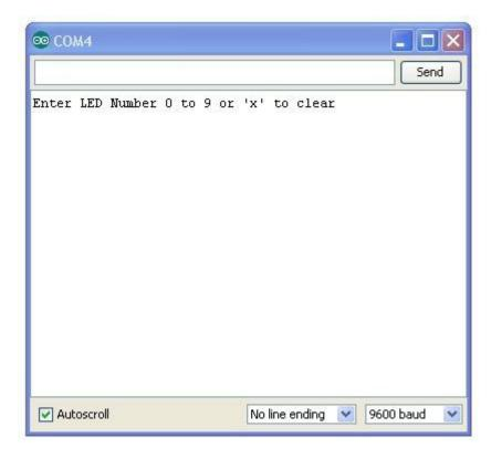
This window is called the Serial Monitor and it is part of the Arduino IDE software. Its job is to allow you to both send messages from your computer to an Arduino board (over USB) and also to receive messages from the Arduino.
