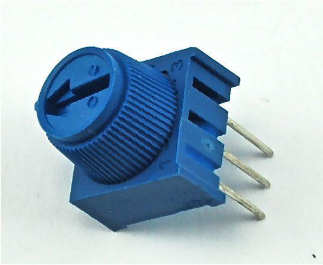
10 kΩ variable resistor (pot)
