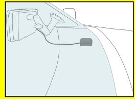
2. For better signal, place antenna as close as possible to the windshield
