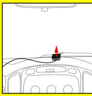
1. Use magnet to attach antenna to a level part of the center of the dash board
