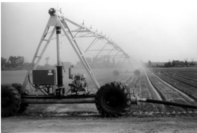
Figure 6. Hose-fed linear move irrigation system
