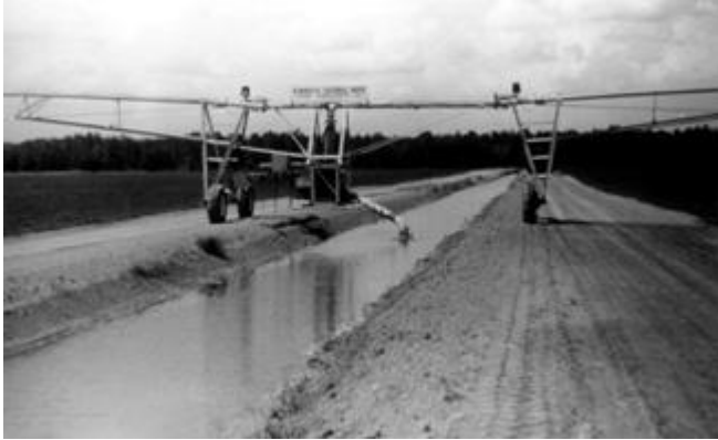
Figure 5. Ditch-fed linear move irrigation system
