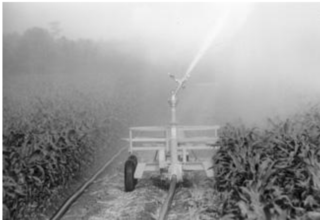
Figure 7. Cable-tow traveler irrigation system
