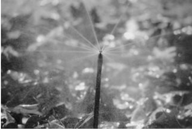
Figure 13. Example of a micro-sprinkler
