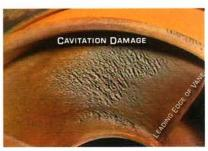
At rates of flow greater than allowed, the NPSH required increases substantially and cavitation damage of the impeller and high vibration levels can become problems.
