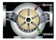
Positive displacement of liquid can also be accomplished by rotary devices such as a vane type rotary pump.
