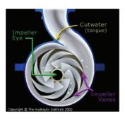
Pumps add energy to the liquid by either of two methods, centrifugal force or positive displacement. Centrifugal pumps use a rotating impeller with multiple vanes as shown here. The liquid enters the impeller axially at the smaller diameter, called the impeller eye, and progresses radially between the vanes until it exits at the outside diameter.
