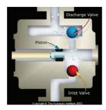
Positive displacement pumps impart energy by applying mechanical force directly to the liquid. One design uses a reciprocating piston to force the liquid out of a closed cylinder.
