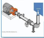
Many process pump applications have pumps connected to a tank above ground, called flooded suction, and discharge into another tank at higher level or pressure.
