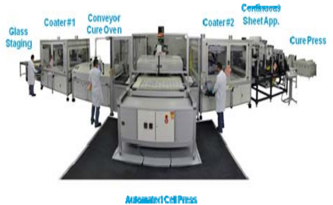
Figure 5: Dow Corning® PV-6100 Cell Encapsulant Series Module Assembly Pilot Line Freeland, Michigan, USA
