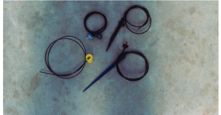
Figure 18. Various irrigation emitters, including button emitters and spray stakes.
