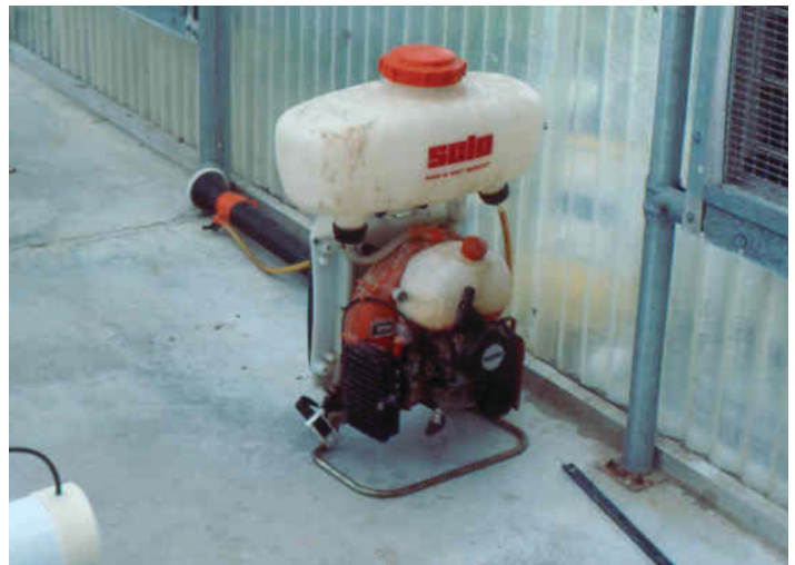
Figure 31. Motorized, backpack sprayer for applying pesticides.
