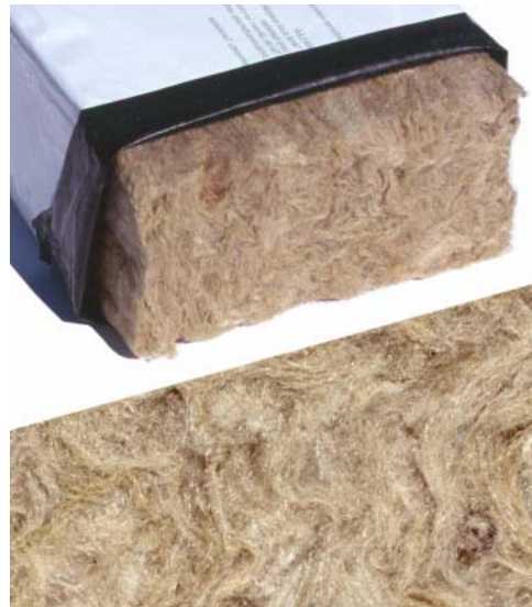
Rockwool - rockwool comes in cubes, slabs and loose bales. It has a very good air to water holding capacity and is used heavily by the commercial greenhouse industry.
