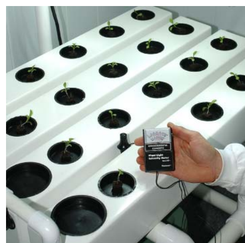
When lighting an indoor garden it is of particular value to establish an evenly lit area. A portable light meter can be of great help in this regard.
