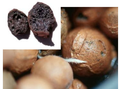
Close-up view of young tomato root as it grows into expanded clay aggregate. Inset shows inner porosity of LECA stone.
