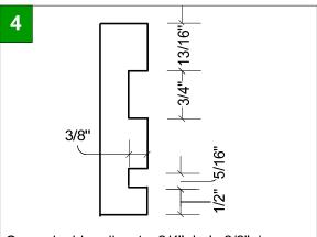
On each side rail, cut a 3/4" dado 3/8" deep and 13/16" from the top. Cut a second dado 5/ 16" wide and 1/8" deep 1/2" from the bottom.
