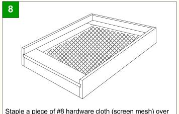
Staple a piece of #8 hardware cloth (screen mesh) over the opening on the top of the frame. Fold the edges over to make a 1/2-inch seam to cover the sharp wire stubs.
