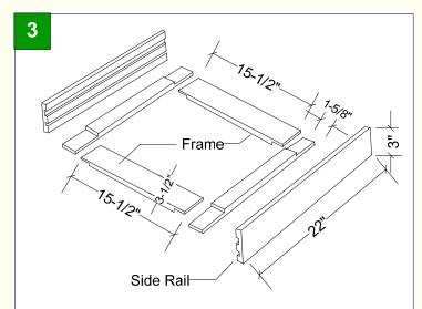
From 1x4 pine, cut two side rails 22" long and 3" wide. For the frame, cut 2 pieces 15-1/2" long by 3-1/2" wide and 2 pieces 22" long by 1-5/8" wide.
