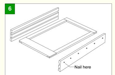
Glue and nail the frame into the 3/4" dados on the side rails. The wide board on the frame goes toward the front, as shown.
