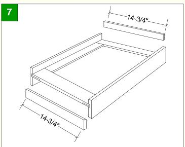
Glue and nail two fillers, each 14-3/4" long, made out of scrap 1x4. One goes in front below the frame and the other goes in back above the frame. Theses fill in the gap between the frame and the bottom (or top) of the rails.
