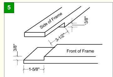
The bottom board frame is joined by simple lap joints. Take care to insure that each lap is 3/8" deep.
