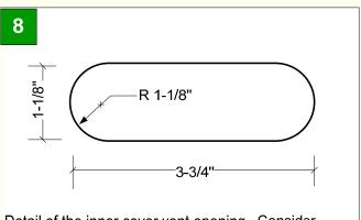
Detail of the inner cover vent opening. Consider making a template and then use a router to create the opening.
