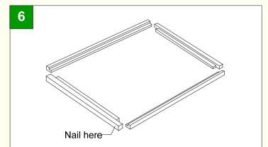
Glue and assemble the frame, checking for square. Use two 1-1/2" 18 ga. nails on each corner. You may need to pre-drill the nail holes to prevent splitting if using larger diameter nails.
