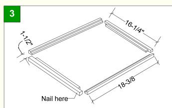
The frame is made from 3/4" stock that is 1-1/2" wide. Two end pieces 16-1/4" long and two side pieces 18-3/8" long are required. The inside top edge of the frame has a 3/4" rabbet that is the same depth as the cover stock.
