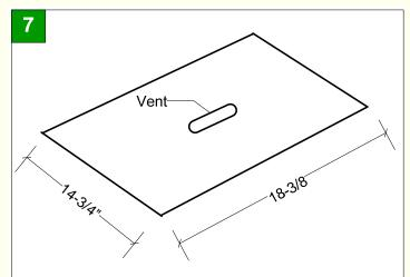
The cover is 14-3/4" by 18-3/8"cut from 1/4-inch plywood. The vent opening is 1-1/8" by 3-3/4" with rounded end.
