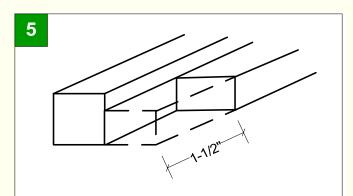
From the end pieces, remove 1-1/2" of the ledge formed by the rabbet. This will allow the end to butt up against the side creating a rebate joint.
