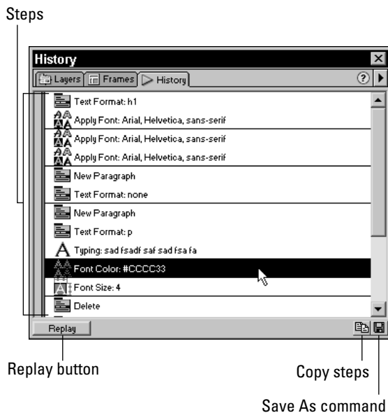
Figure 3-17: Undo or redo any series of actions by moving the slider in the History panel.
