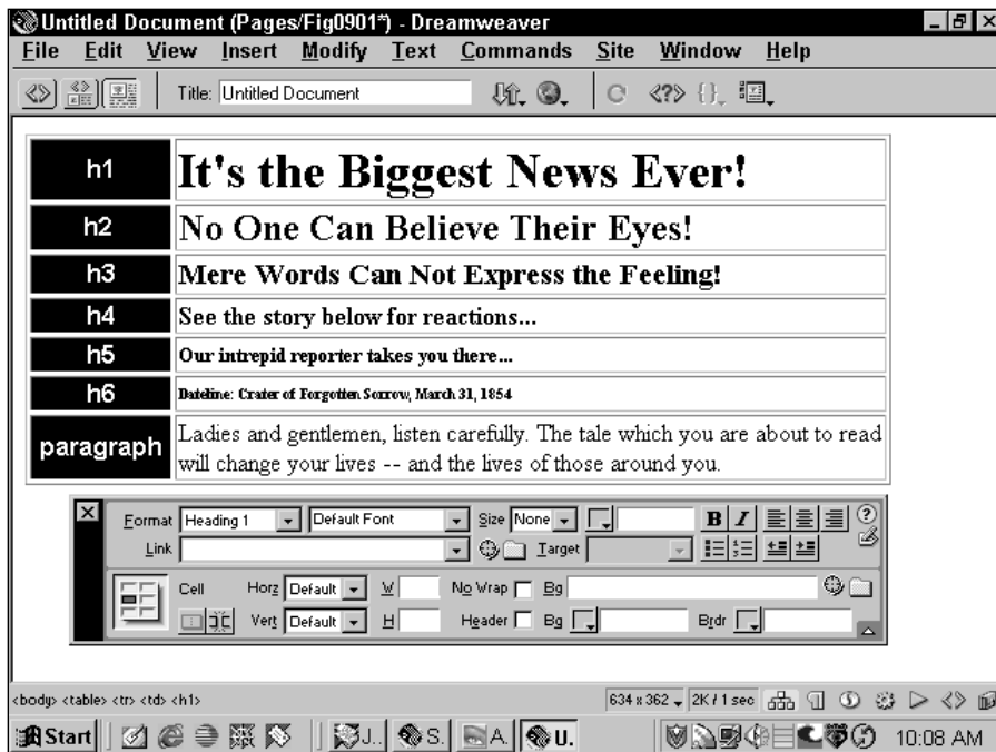
Figure 9-1: Standard HTML enables you to use up to six different size headings.
