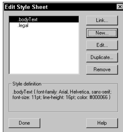
Figure 27-3: The Edit Style Sheet dialog box lists and defines any given style, in addition to presenting several command buttons for creating and managing styles.
