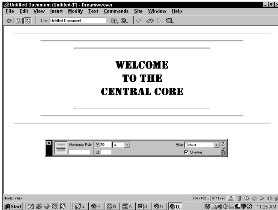
Figure 10-10: The Horizontal Rule Property Inspector controls the width, height, and alignment for these HTML lines.
