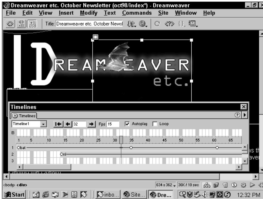
Figure 1-7: Use the Timelines panel to animate objects in layers using Dreamweaver’s advanced Dynamic HTML features.
