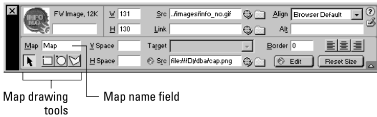
Figure 14-1: From the Image Property Inspector, select the image map tools to draw hotspots directly on graphics within Dreamweaver.
