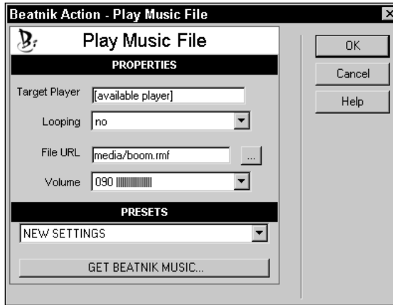
Figure 25-9: Start any RMF or MIDI file through the Play Music File behavior.
