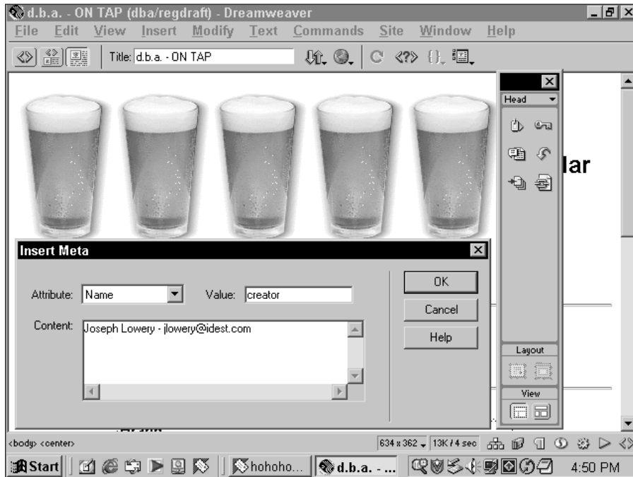
Figure 8-3: The Meta object enables you to enter a full range of <meta> tags in the <head> section of your Web page.
