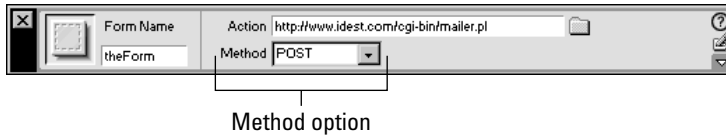
Figure 17-3: Use the POST method to send information via a form to most CGI programs.
