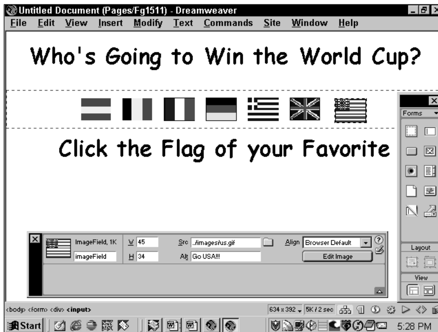
Figure 15-11: Each flag in this page is not just an image; it's an image field that also acts as a Submit button.
