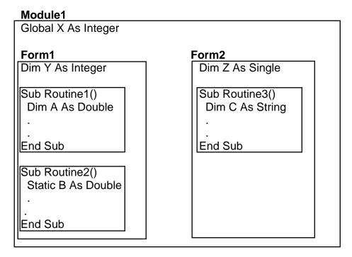
Procedure Routine1 has access to X, Y, and A (loses value upon termination)
