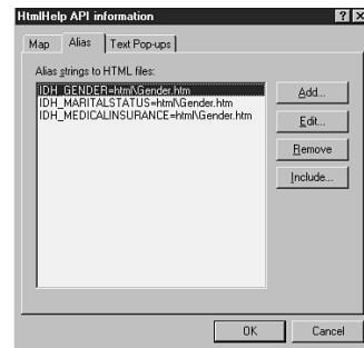
FIGURE 7.29 ▲ The newly created list of topic file-to-constant mappings on the Alias tab of the HTMLHelp API Information dialog box.
