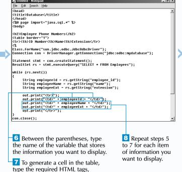
enclosed in quotation marks. Separate each tag and variable with the concatenation operator.
