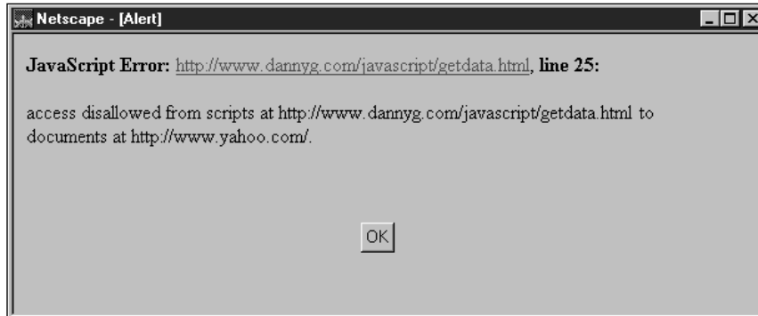
Figure 40-2: Attempting to retrieve a secure property from another server's document yields a script error showing the URLs of the documents containing your script and the secure information.
