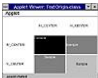
Figure 7-5 A getTextOrigin method to center rendered text within a rectangle horizontally or vertically
