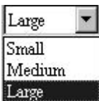
Figure 6-2 Use of a choice button to specify the size of a pizza
