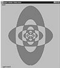
Figure 1-6 Screenshot of Ovals applet, demonstrating the XOR painting mode of the Graphics class
