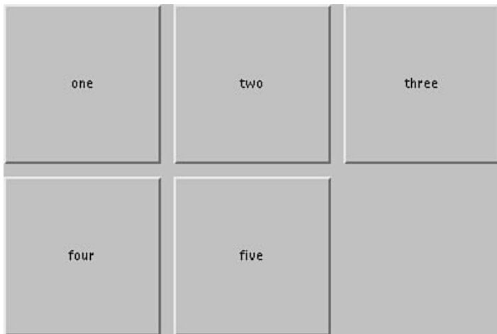
Figure 13.12. Grid layouts with horizontal and vertical gap.
