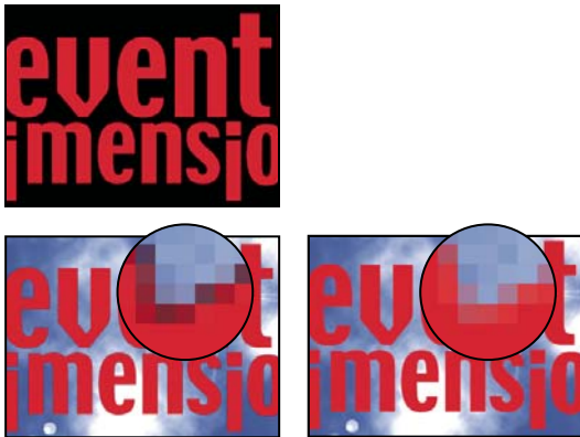
Item with premultiplied channels (top) appears with a black halo when interpreted as Straight-Unmatted (lower-left). When interpreted as Premultiplied-Matte with black specified as background color, halo does not appear (lower-right).
