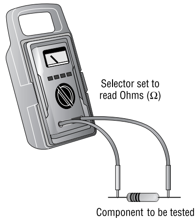
FIGURE 1.22 Connecting a multimeter to measure resistance
