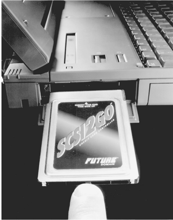
FIGURE 49-1 A PC Card SCSI adapter for mobile computers (copyright © 1995 Future Domain Corporation; reprinted with permission)
