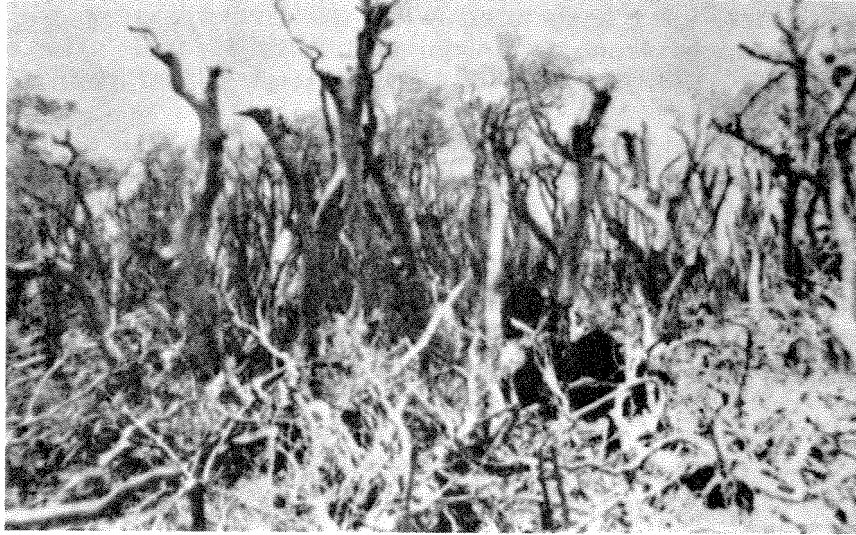
DECIDUOUS FOREST SUBJECTED TO 2.4 PSI FROM A MEGATON -RANGE WEAPON. NOTE EXTENSIVE CROWN BREAKAGE
