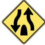
Divided Highway (Road) Ends
