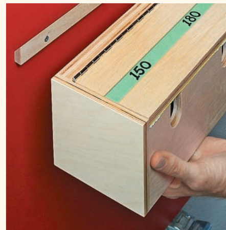
▲ A simple cleat allows you to hang the box in a convenient location, keeping sanding supplies close at hand.
