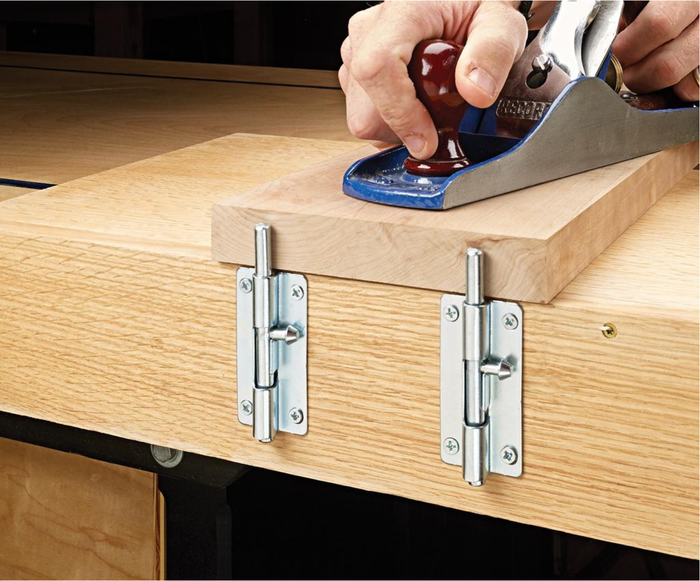
Serge Duclos from Delson, Quebec attaches barrel bolts to the sides of his workbench to serve as additional bench stops.
