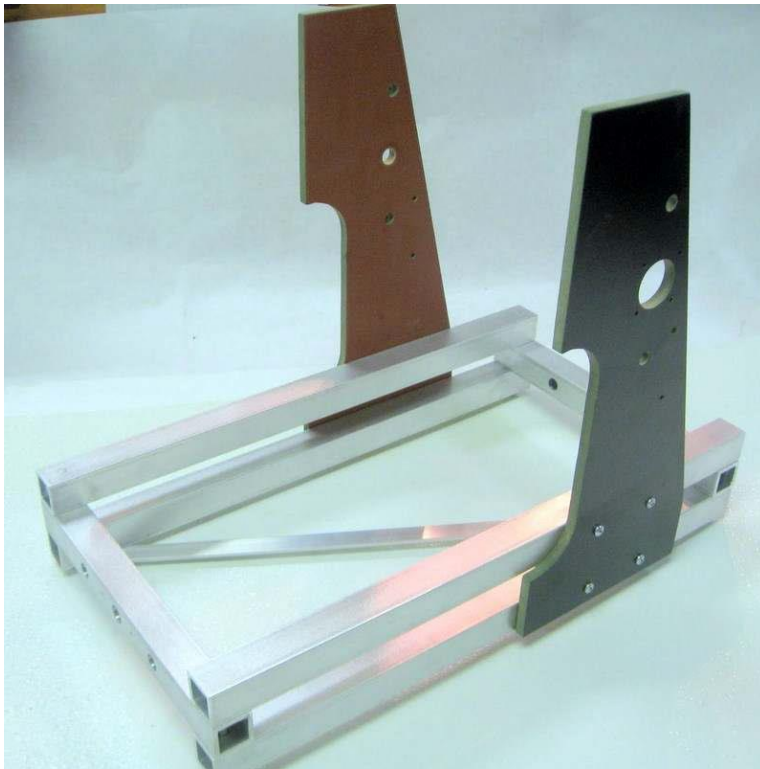
Gantry support uprights attached to chassis
