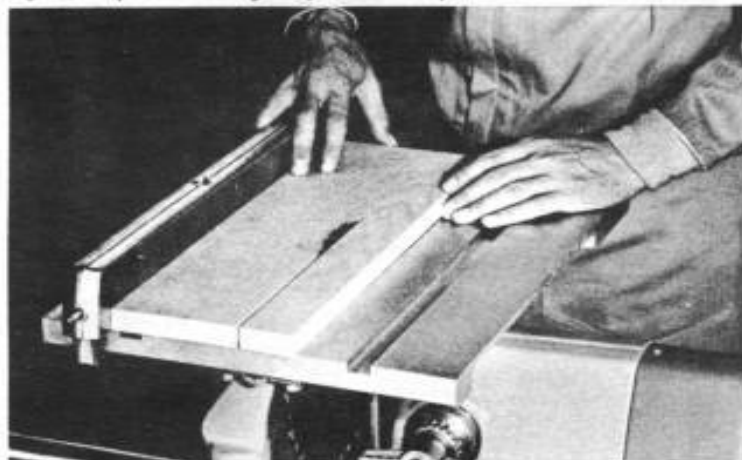
Fig. 20 Hook fingers over fence when ripping
