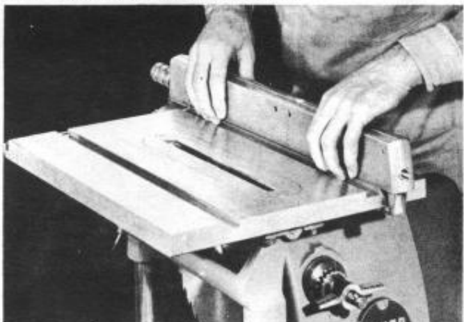
Fig. 9 Rip fence must be parallel with table slots
