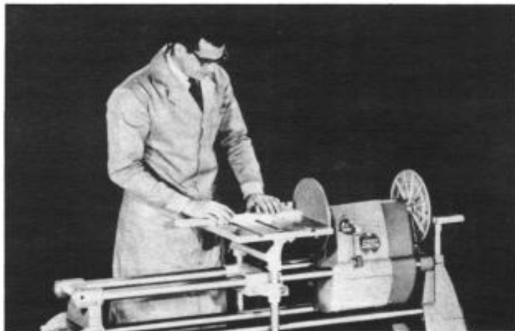
Fig. 59 Dual sanding is possible on SHOPSMITH M5
