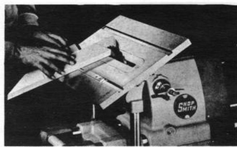
Fig. 25 Compound angle is combination miter and bevel
