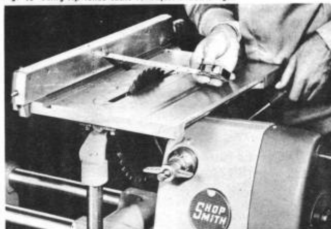
Fig. 16 Using quill feed for blade to fence setting
