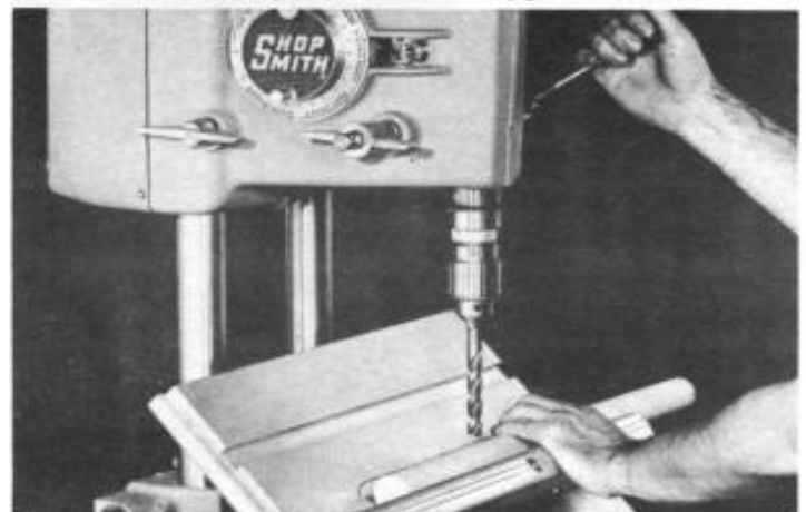
Fig. 44 V-Block jig for drilling round stock
