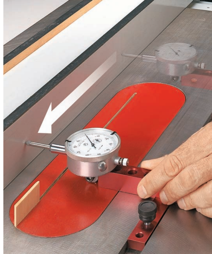
▲ Dead-On Fence. A dial indicator makes it easy to check the front and rear of the rip fence and ensure that it's parallel to the miter slot (and the saw blade).
