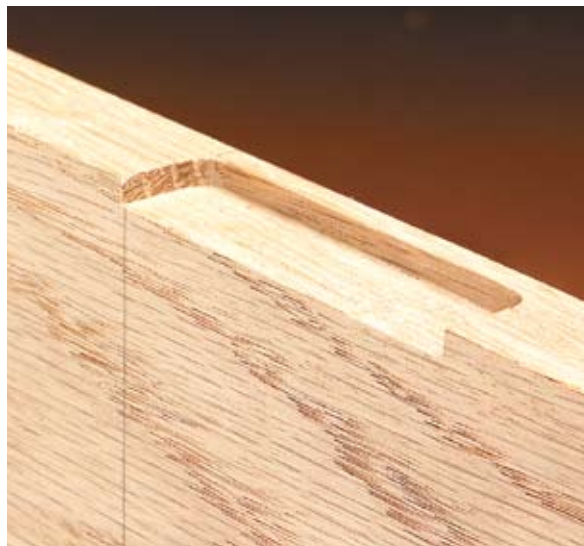
▲ A Mortise for a Hinge. Quick, clean, and accurate describe the mortise you get with a trim router and this hinge mortising jig.
