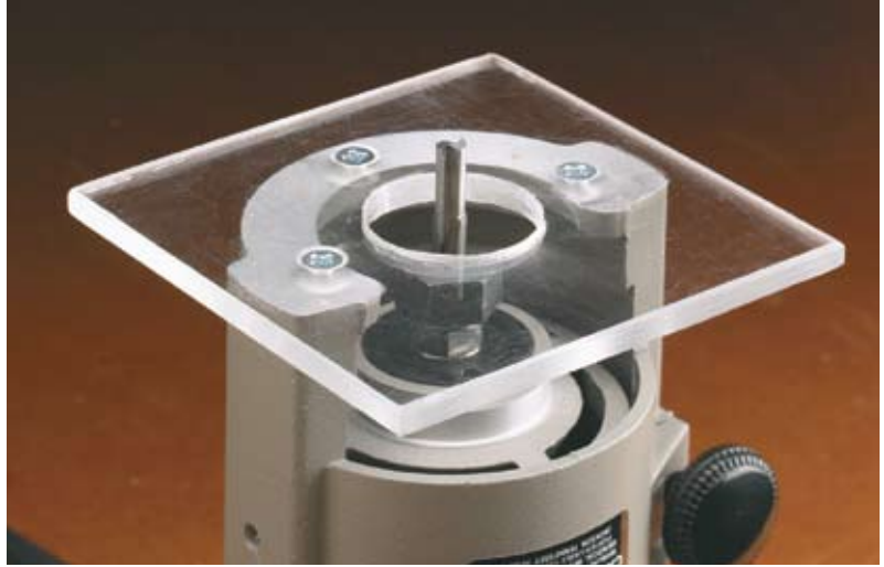
▲ Baseplate. To improve visibility and accuracy while you rout, replace the round baseplate with a square piece of clear plastic.
