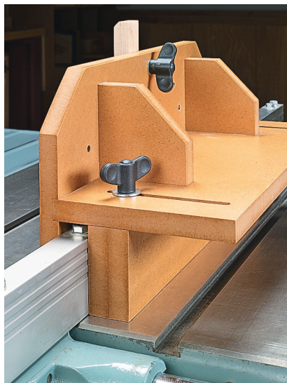
▲ Narrow Fence. There's no need to build a second jig for a narrower fence. The jig adjusts to fit them all.
