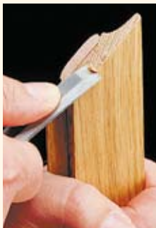
▲ To ensure a tight-fitting miter, you may have to undercut the end of each workpiece slightly.
