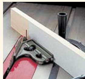
▲ Use the head of a combination square to set the miter gauge at 45°.
