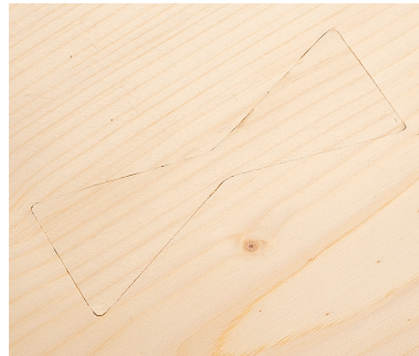
{ An inlaid patch with matching grain solves the problem and is almost undetectable.
