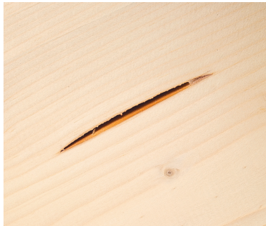
{ A pitch pocket is just one example of a defect that can detract from the look of a project.
