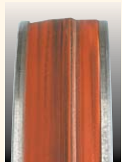
▲ Tire Wear. The ridge on this tire was caused by setting the blade tension too high.
