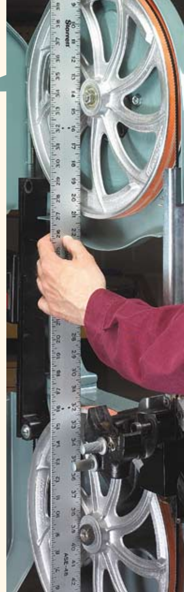
◀ Vertical Wheel Alignment. A long straightedge placed across the top and bottom wheel makes it easy to check the alignment of the wheels.
